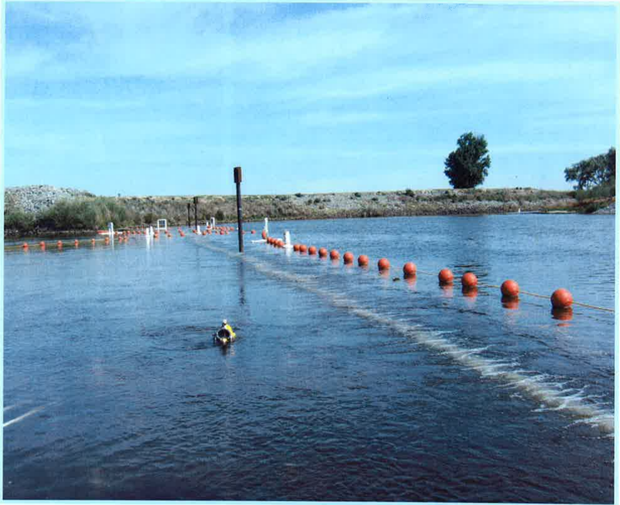
Figure 9. NPB in operation with bubbles breaking surface of river
